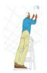
Don't work on the top 3 rungs – Don't work any higher up on this type of stepladder.
