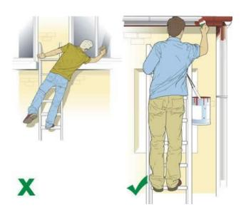
Keeping three points of contact – Ladder showing correct 1 in 4 angle (Securing omitted for clarity).
