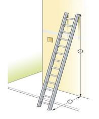
Positioning a leaning ladder safely – Ladder showing correct 1 in 4 angle (Securing omitted for clarity).
