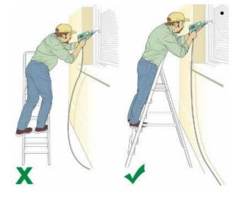
Don't work on the top 3 rungs – Don't work any higher up on this type of stepladder. Always face your work, never work from the side of the ladder.
