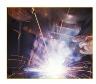
The U.S. Chemical Safety & Hazard Investigation Board has identified more than 60 fatalities since 1990 due to explosions and fires from hot work activities on tanks. Hot work is defined as "work involving burning, grinding, welding, gouging or a similar operation that is capable of initiating fires or explosions."
